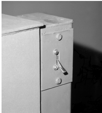
Figure 10: Powered rear access ladder switch
